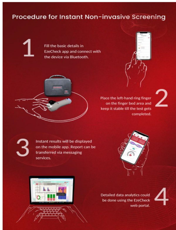
Figure 2. Representation of the process involved for conducting the Non-invasive Haemoglobin test using the EzeCheck device.
