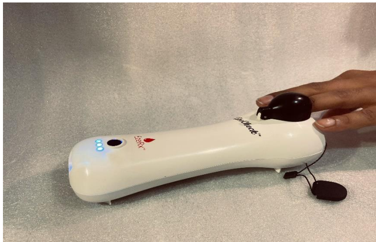
Fig:1 Non-invasive haemoglobin screening device- EzeCheck
